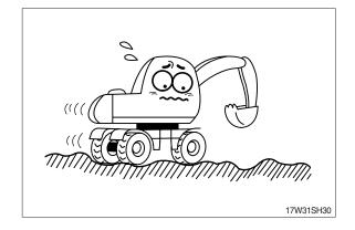
When operating in water or when crossing shallow, check the bed soil condition and depth and flow speed of water, then proceed taking care that water is not above axle center.
