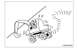
The engine angularity limits are 35 degree. Do not operate by more than the engine limits in any case.
